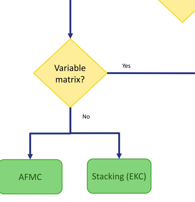
Analyte focusing by micelle collapse -The sample is mixed with micelles, the BGE is micelle-free. The micelles collapse when meeting the solvent or the BGE
